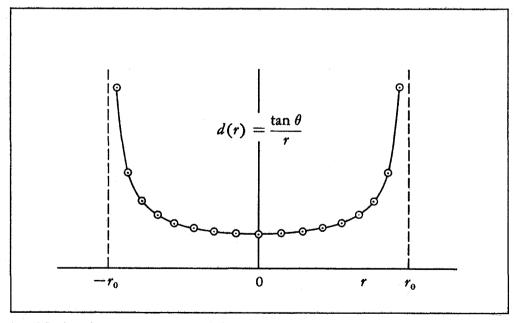
(6) Notice that  $\tan \theta$  is an odd function of  $\theta$ , and that  $\theta$  is an odd function of r. As a result,  $\tan \theta$  is an odd function of r, and so d(r) must be an even function of r. If the  $r(\theta)$  relationship is extrapolated smoothly to  $r(90^\circ) = r_0$ , then d(r) will have simple poles at  $\pm r_0$ .
