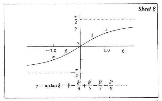
(28) Sometimes it is advisable merely to note that a function is even or odd in choosing a suitable parametric form. An approximation so made to hold over (0, 1) then automatically holds over (-1, 1).
