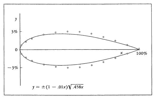
(13) Then we solved for y in terms of x and prefaced the resulting right member by a factor (1 - .01x) to bring the curve down to zero at x = 100%. As the trailing edge doesn't exactly come to a point, this is a slight violation of the data.
