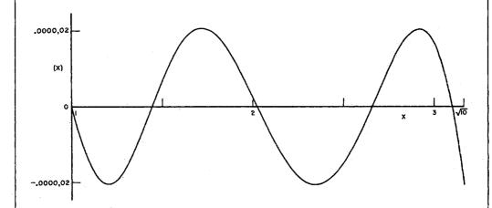
$$\log_{10}^* X = \frac{1}{2} + C_1 \left( \frac{X - \sqrt{10}}{X + \sqrt{10}} \right) + C_3 \left( \frac{X - \sqrt{10}}{X + \sqrt{10}} \right)^3 + \dots + C_7 \left( \frac{X - \sqrt{10}}{X + \sqrt{10}} \right)^7.$$
