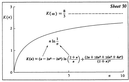
(31) A very simple approximation to K(n) over  $(0, \infty)$  was required for use on a high-speed digital computing machine. If at all possible, we were to obtain a rational fit, but observe: K(n) has an infinite derivative at n = 0!
