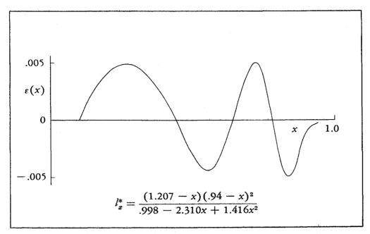
(19) A second requirement then appears to be a nearly equal quadratic term downstairs that can cancel the early effect of the  $(.94 - x)^2$  term upstairs and yet not detract from the ability of this latter term to give the proper shape to the curve near the end of the table.
