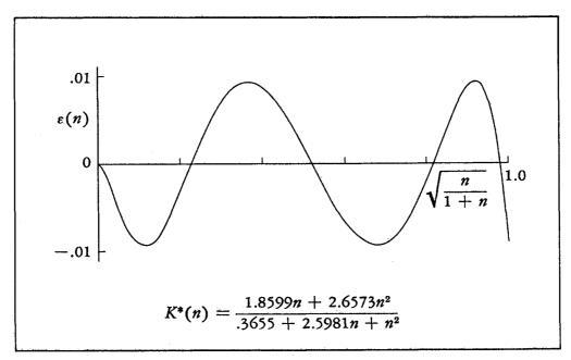
(32) And yet, despite the apparent difficulty of the task, a quadratic over a quadratic gave us a fit good to about .01, and a cubic over a cubic gave a fit good to about .001. Perhaps the indicated singularity is not quite so bad as a  $\sqrt{n}$  singularity would be.
