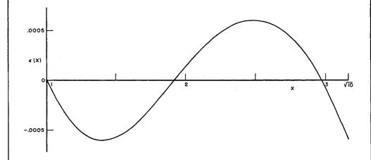
$$\log_{10}^* X = \frac{1}{2} + C_1 \left( \frac{X - \sqrt{10}}{X + \sqrt{10}} \right) + C_3 \left( \frac{X - \sqrt{10}}{X + \sqrt{10}} \right)^3.$$
