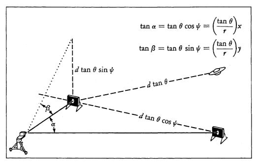
(13) The lens system is assumed to introduce no distortion of angle about the optical axis. The big problem is that of converting film coordinates x and y into angular space coordinates  $\alpha$  and  $\beta$ .
