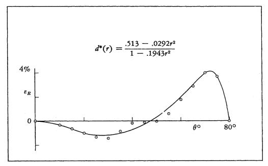
(8) As  $r_0$  is unknown, we replaced the quantity  $r_0^{-2}$  by the parameter  $b_2$ . In our first attempt at fitting, we tried just two terms upstairs. To obtain additional points on the error curve, we interpolated midvalues of  $r(\theta)$  and computed corresponding d(r) values.
