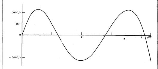
$$\log_{10}^* X = \frac{1}{2} + C_1 \left( \frac{X - \sqrt{10}}{X + \sqrt{10}} \right) + C_3 \left( \frac{X - \sqrt{10}}{X + \sqrt{10}} \right)^3 + C_5 \left( \frac{X - \sqrt{10}}{X + \sqrt{10}} \right)^5.$$
