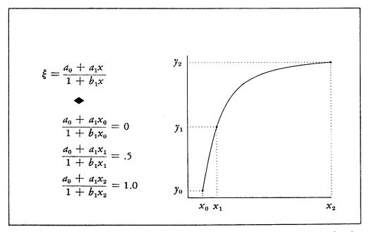
(23) Often we run into curves that may be made quite polynomial-like by the use of the simple rational transformation  $x \to \xi$  defined above. To determine suitable parameter values, we divide the vertical range of variation into two (roughly) equal parts.
