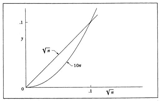
(33) This is easily seen to be the case, and the fact is illustrated in the pair of diagrams on this page. Against a  $\sqrt{n}$  horizontal scale, the function  $y = \sqrt{n}$  is a straight line with unit slope, whereas the function  $y = -n \ln n$  is a curve with zero slope at the origin.
