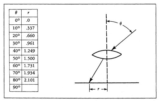
(3) A photograph is taken and measured to yield data giving image distance r as a function of entering-ray angle  $\theta$ . The distance r is measured from the point on the film intersected by the optical axis. A sample of such calibrating data was given to us by Mr. Lowe.
