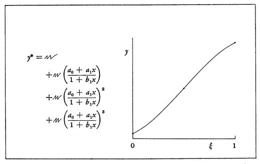
(24) We then require that  $x_0$ ,  $x_1$ , and  $x_2$  transform to equally spaced  $\xi$  values of, say, 0, .5, and 1.0. The transformed curve is then approximated by a polynomial in  $\xi$  in the usual fashion.
