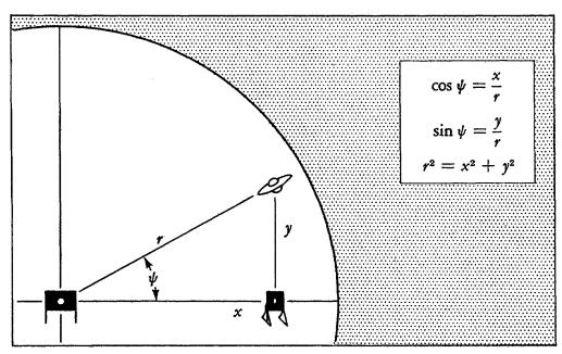
(12) And this is the remainder of the story: Coordinates x and y of the image of an object in space are read from the film. To clarify the geometry, we consider the space object to be vertically above the ground target on the right.
