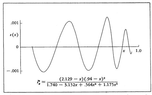
(20) A final requirement appears to be a linear term upstairs that can give the curve its required early linear appearance. Further terms then serve to supply added flexibility; but we may ask, at this point, "How really good are these data, anyway?"
