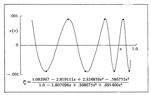
(16) We attempted to fit a polynomial of second degree in x over a polynomial of second degree in x to  $l_x$  but were unable to level the error curve. Then we tried a cubic over cubic and obtained the rather remarkable approximation above.
