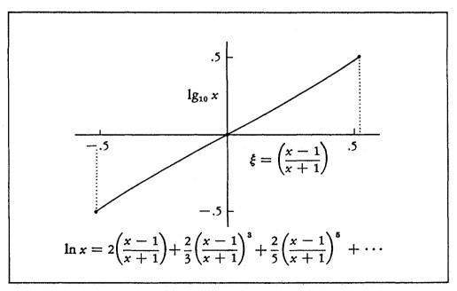
(26) But now let us introduce the transformation  $\xi(x) = (x-1)/(x+1)$ . When plotted against the new variable,  $\xi$ , the three points become equally spaced horizontally as well as vertically, and the curve is now quite flat.
