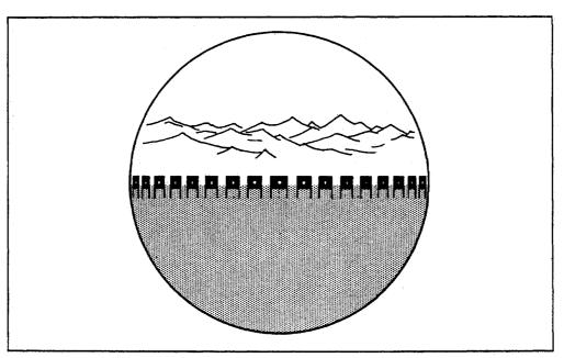
(2) To calibrate a scoring camera, a target array is set up and is photographed by the camera to be calibrated. The optical axis of the lens system is centered on the middle target of the array.
