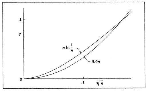
(34) Both the quadratic over quadratic and the cubic over cubic forms behave like An for small n, and against a  $\sqrt{n}$  scale An plots as a parabola with zero slope at the origin.
