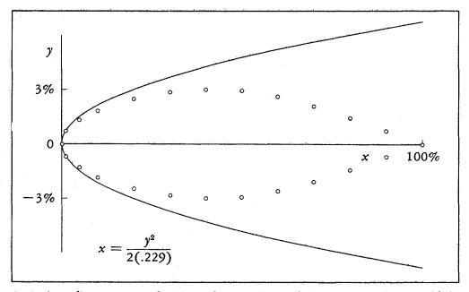
(12) As a first step, we determined a simple parabola  $x = Ay^2$  that would fit a small region of the leading edge well. For this purpose we chose A so that the parabola would have the proper curvature at the origin.
